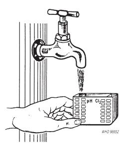
**B.** Add tablet or liquid reagent and mix thoroughly to dissolve. This may require the crushing of the tablet with a clean glass rod.
